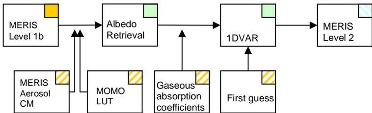
Figure 1: Flow chart for the MERIS L2 processor. Input data is marked in orange (orange shaded: higher level input data), products are marked in blue (blue shaded: instantaneous level 2 products) and software development is marked in green. (CM: cloud mask, LUT: Look-up table)
